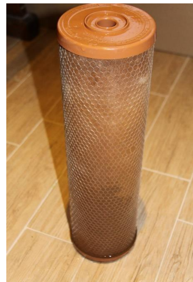
Photo of the rust saturating a non-replaced cartridge (due to the galvanization of the pipes of the water supply company)
