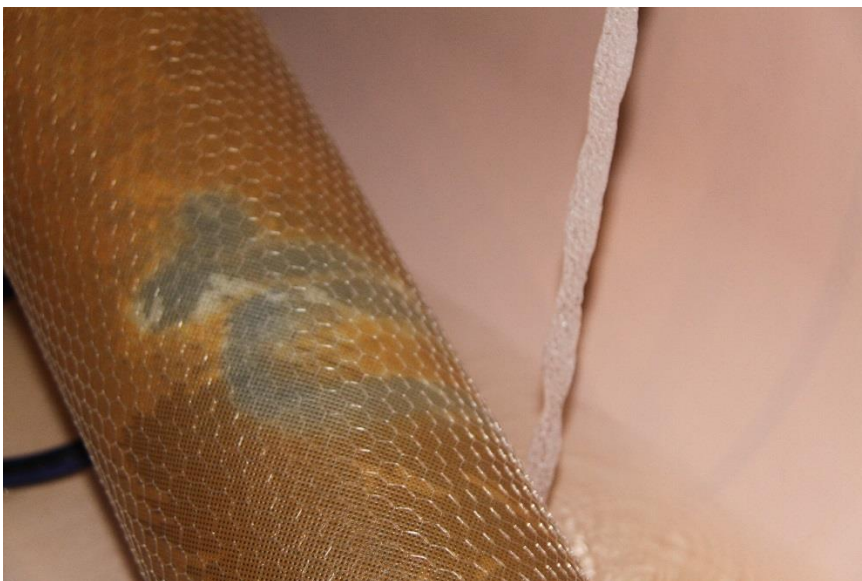
Photo of the rust saturating a non-replaced cartridge (due to the galvanization of the pipes of the water supply company)
