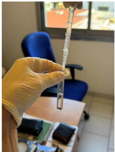
Figure 8 Test tube: Borosilicate test tubes low fluorescence interference
